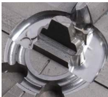
Fathom tool after sinker EDM and polishing operations
