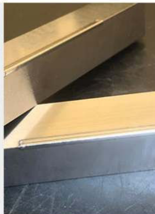
Mantle’s printed H13 part post laser welding
