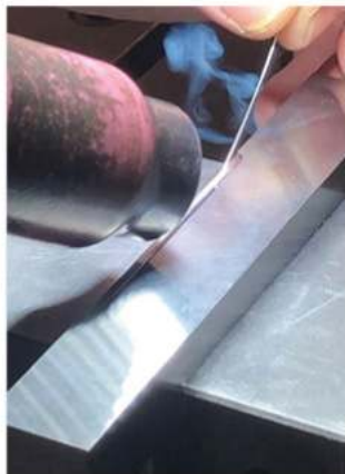
Laser welding of the Mantle printed H13 part
