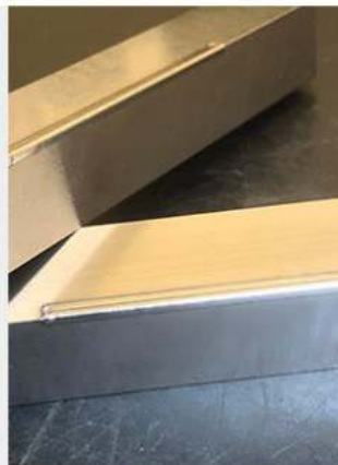
Mantle’s printed H13 part post laser welding
