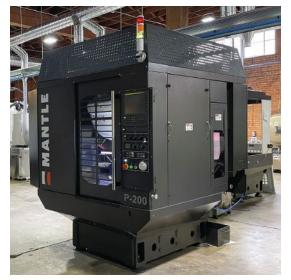
The Mantle process rapidly 3D prints and machines mold tooling made from H13 or P20 steel, using a machining center that has been modified to incorporate the metal paste layering.
