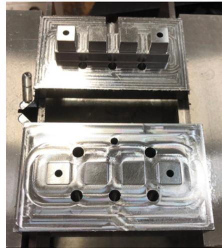
Fig: Mold inserts machined side by side
