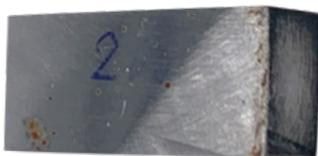
P20 Tool Steel after Corrosion Testing
